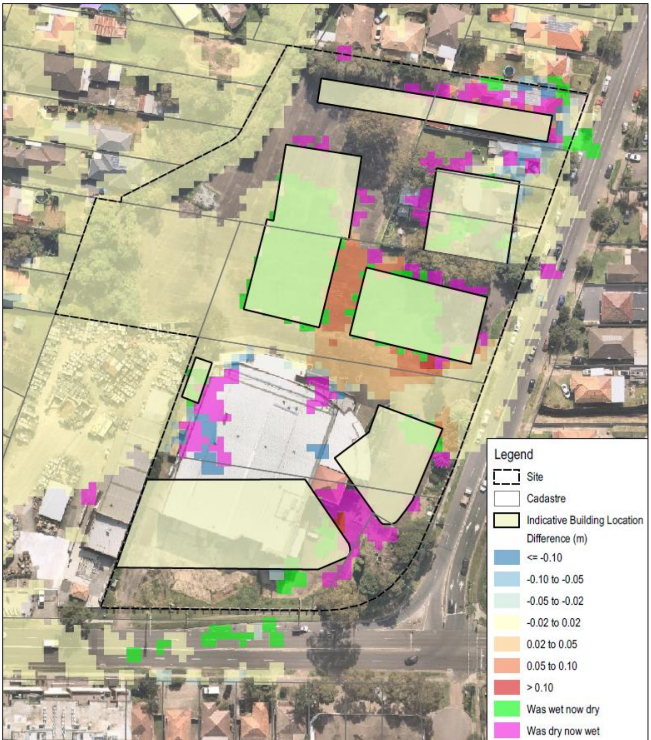
Figure 4-5 Flood Impacts - Post-Development Less Existing – 1% AEP Event
