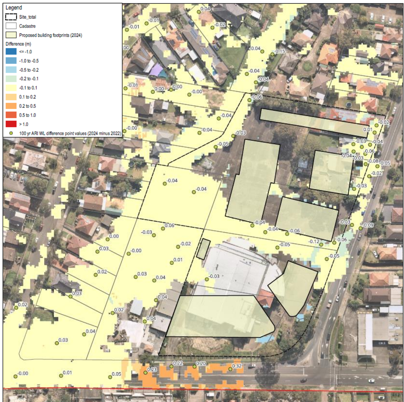
Figure 4-3 Water Level Differences – Sensitivity - Revised Less Original Model - 1% AEP for Post-development Scenario
